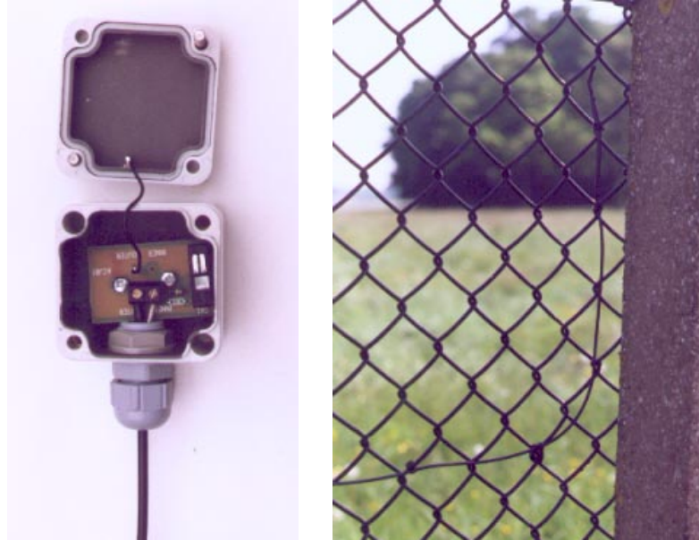
Figure 15 End of zone termination.
