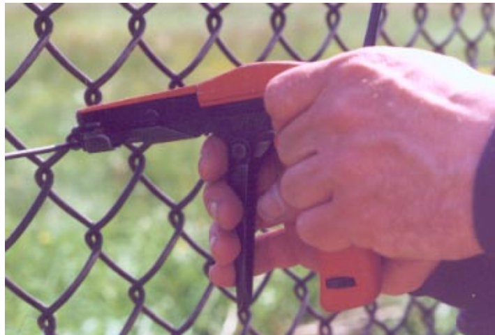
Figure 11 Using a tie wrap gun to tighten and trim cable ties.
